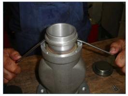
**2)** Use two tools one opposite to the other to lever and remove the valve inlet bushing.
