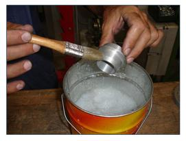
**5)** Lubricate the outer side of the bushing using only silicone grease.
