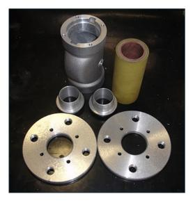
**1)** Prepare the components: body - bushings - flanges - sleeve.
