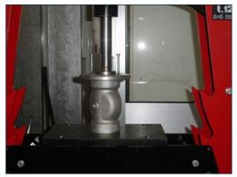
8) Using a press (or the forks of a forklift) to abut the bushingflange unit to the body. Tighten the flange to the body by means of the holes, and be reminded to replace the two long screws used as pins with suitable screws to fasten the flange.
