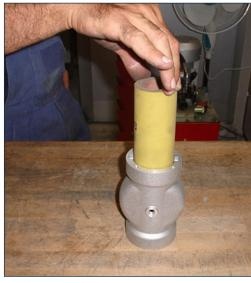
**2)** Fit the sleeve inside the valve body. In case it doesn't slip in easily, grease the inner side of the body with silicone grease.
