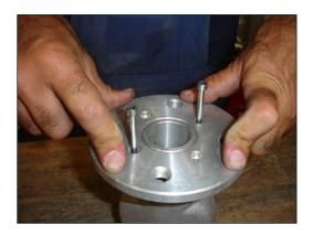
7) Insert the flange in the bushing seat. Use two long screws positioned 180 degrees from each other as centring pins, so that the holes of the flange match the holes of the body, prevent the flange from rotating.
