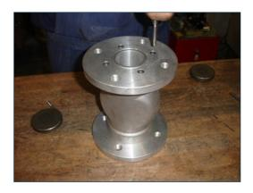
**1)** Use an Allen key to unscrew the screws of the inlet flange. Once free, you can extract it manually.
