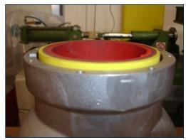
**4)** Make sure the sleeve protrudes from the upper edge of the body of a few millimetres (do not exceed 2 mm).
