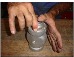
**6)** Insert the first bushing in the sleeve; make sure it slide sin uniformly.
